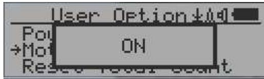
GMC-320 has motion detection feature. It can detect unit movement, upside down, single tap and double tap. Turn off the motion detection disables all motion related features.
