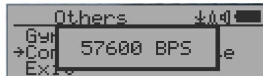
This Geiger counter serial communication baud rate is selectable from following value: 1200,2400,4800,9600,14400,19200,28800, 38400,57600,115200. Press S4 key changes baud rate.
