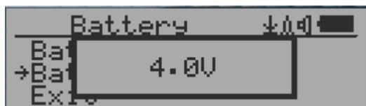
Select Battery submenu and Battery item for checking the current battery voltage.
